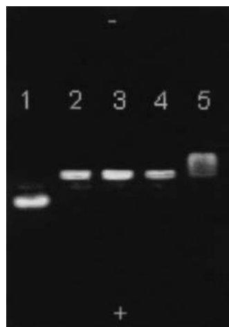
Fig. 2. Agarose gel electrophoresis of nanoemulsion particles and their complexes with p-PLL stained with Nile Red (Lane 1: nanoemulsion; Lane 2 to Lane 5 were the complex of nanoemulsion and p-PLL with the ratio of p-PLL to triolein to be 0.125:1, 0.25:1, 0.5:1, and 1:1 respectively).
